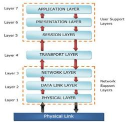
The physical layer, data link layer and the network layer are the network support layers. The layers manage a physical transfer of data from one device to another. Session layer, presentation layer, and application layer are the user support layers. These layers allow communication among unrelated software in dissimilar environments. Transport layer links the two groups.
